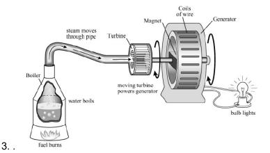
The diagram above shows how energy is transformed in a power plant. During this entire process, energy is transferred from one form to another several times. Describe **four** energy changes that occur during the process.
